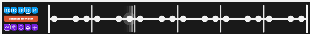
Figure 5: A stave with the generated nodes. Note how the algorithm has chosen to generate a unique pattern of nodes over a single bar, and the remaining bars repeat the first bar in strophic form. The setting buttons for the stave are also visible on the left.
